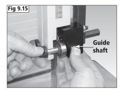
The rear guide must now be set in the correct position. Loosen the rear guide lock shown in **Fig 9.14** and position the guide by moving the guide shaft as shown in **Fig 9.16**.
